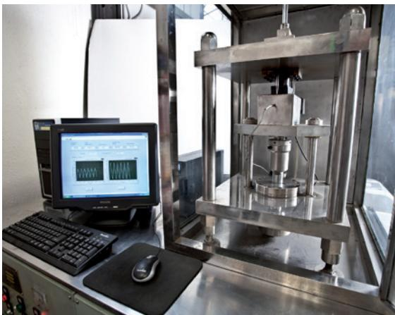
• **Compression test** during which is evaluate the deformation of braking materials subject to a pre determined specific pressure. The value noted must not exceed 2% of the initial thickness during tests at room temperature and do not exceed 5% of the initial thickness during tests at 400°C.
